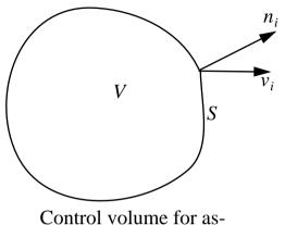
Control volume for assessing conservation of mass. Consider the rate of change of mass within a fixed volume. This changes as a result of the mass flow through the bounding surface.
