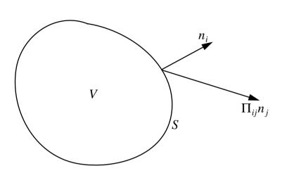
Consider now the rate of change of momentum within a volume. This decreases as a result of the flux of momentum through the bounding surface and increases as the result of body forces (in our case gravity) acting on the volume. Let
