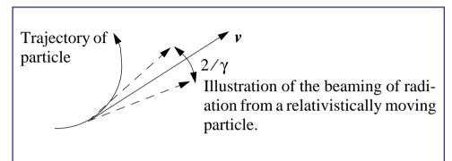
Note the factor  $(1 - \beta \cdot n')^{-3}$  in the expression for the electric field. When  $1 - \beta' \cdot n' \approx 0$  the contribution to the electric field is large; this occurs when  $\beta' \cdot n' \approx 1$ , i.e. when the angle between the velocity and the unit vector from the retarded point to the field point is approximately zero.
