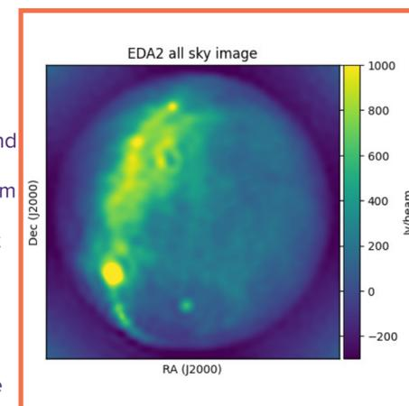
All-sky simulation with the EDA2 instrument using the WODEN simulator tool. WODEN's ability to simulate accurate all-sky images allows the MWA EoR project to test its data analysis tools (credit: Dr Jack Line).
