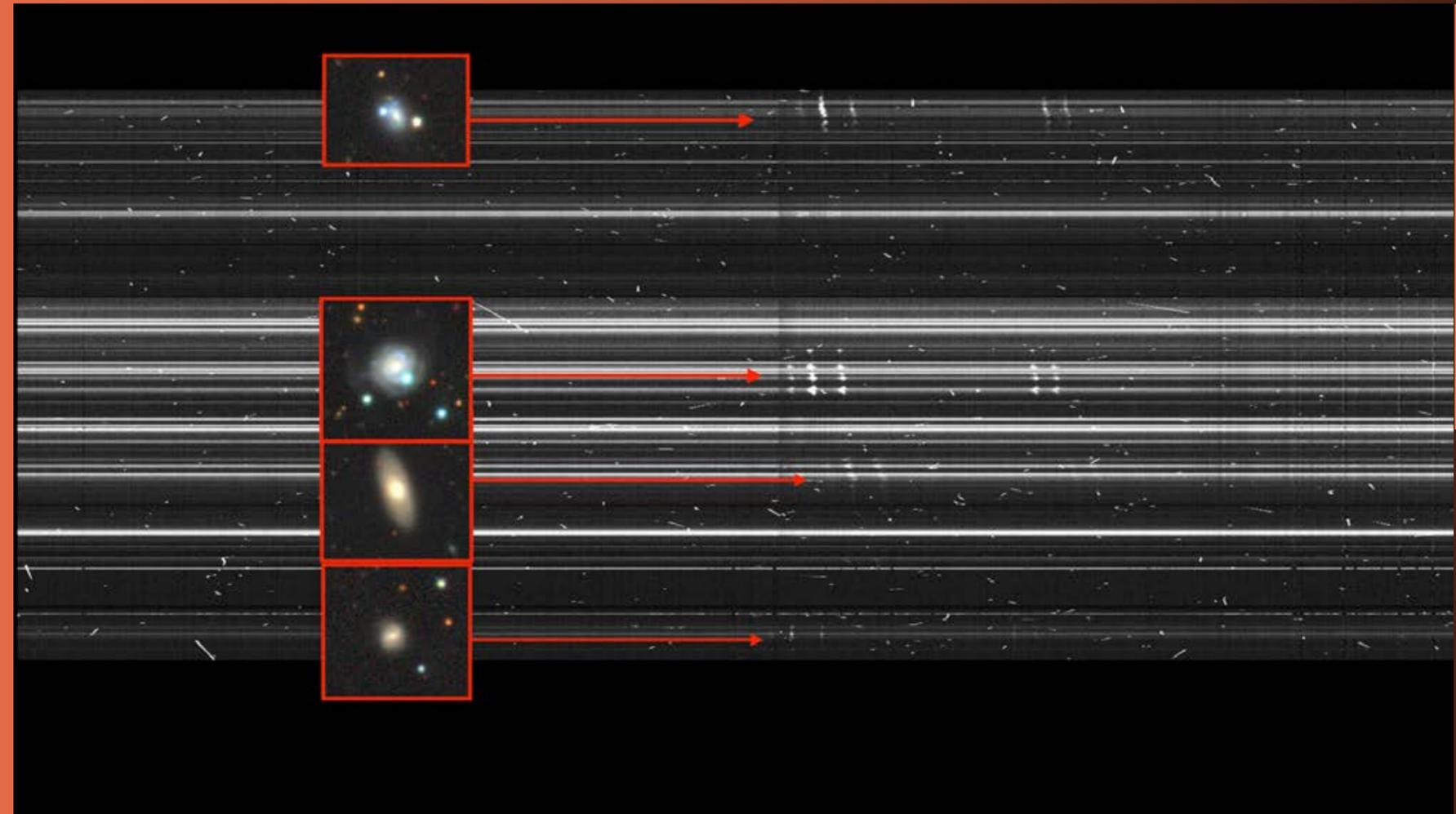
Figure 18: The first galaxy data from the Hector instrument in "row-stacked spectra" format. Each horizontal line is the spectrum from a single optical fibre (blue to the right, red to the left). Groups of fibres target galaxies. The near vertical lines that show small horizontal shifts are gas emission lines, with the shifts due to the rotation of the galaxies being observed. Example images of the galaxies being targeted are shown in the red boxes. Image Credit: Madusha Gunawardhana.
