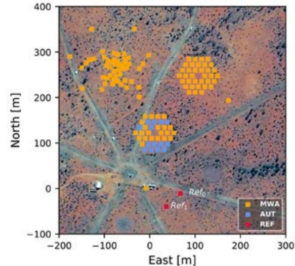
Figure 3: Publication no. 38 - The positions of the AUTs (blue) and the Reference antennas (red). The ochre points represent the rest of the compact core of the MWA.
