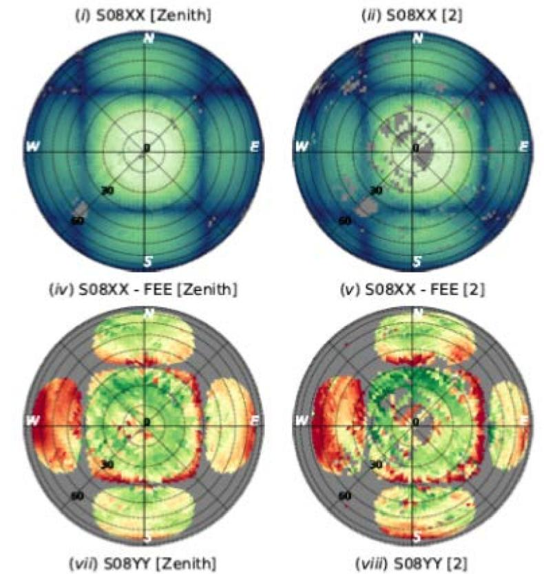
Figure 8: MWA primary beam sky response, mapped via passes over the array of an Orbcomm satellite (top), and difference compared with model (bottom). Chokshi et al 2021, "Dual Polarization Measurements of MWA Beampatterns at 137 MHz", Monthly Notices of the Royal Astronomical Society, Volume 502, Issue 2, pp.1990-2004
