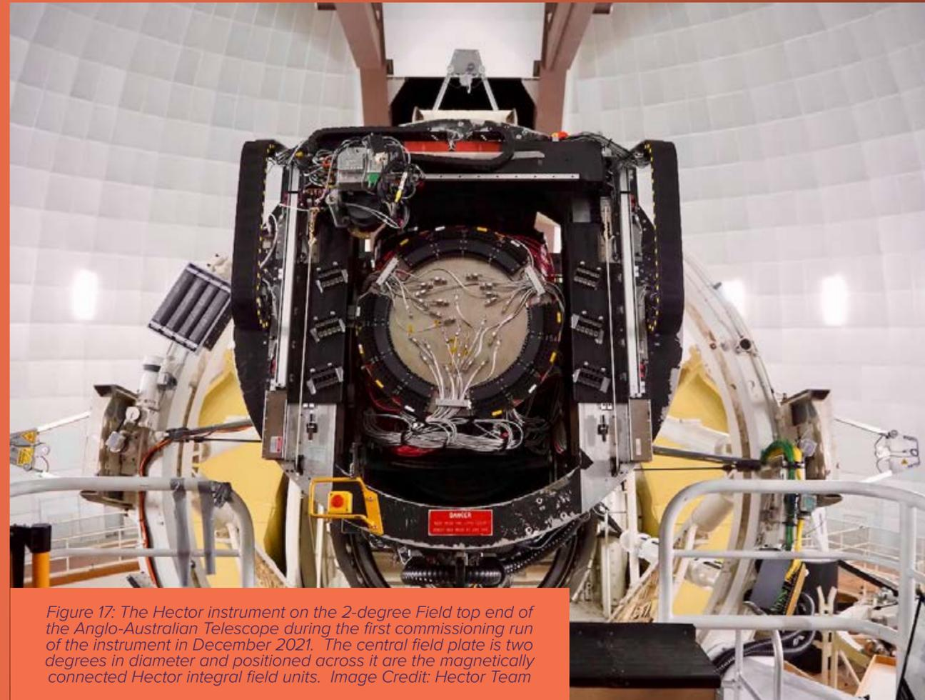
Figure 17: The Hector instrument on the 2-degree Field top end of the Anglo-Australian Telescope during the first commissioning run of the instrument in December 2021. The central field plate is two degrees in diameter and positioned across it are the magnetically connected Hector integral field units. Image Credit: Hector Team
