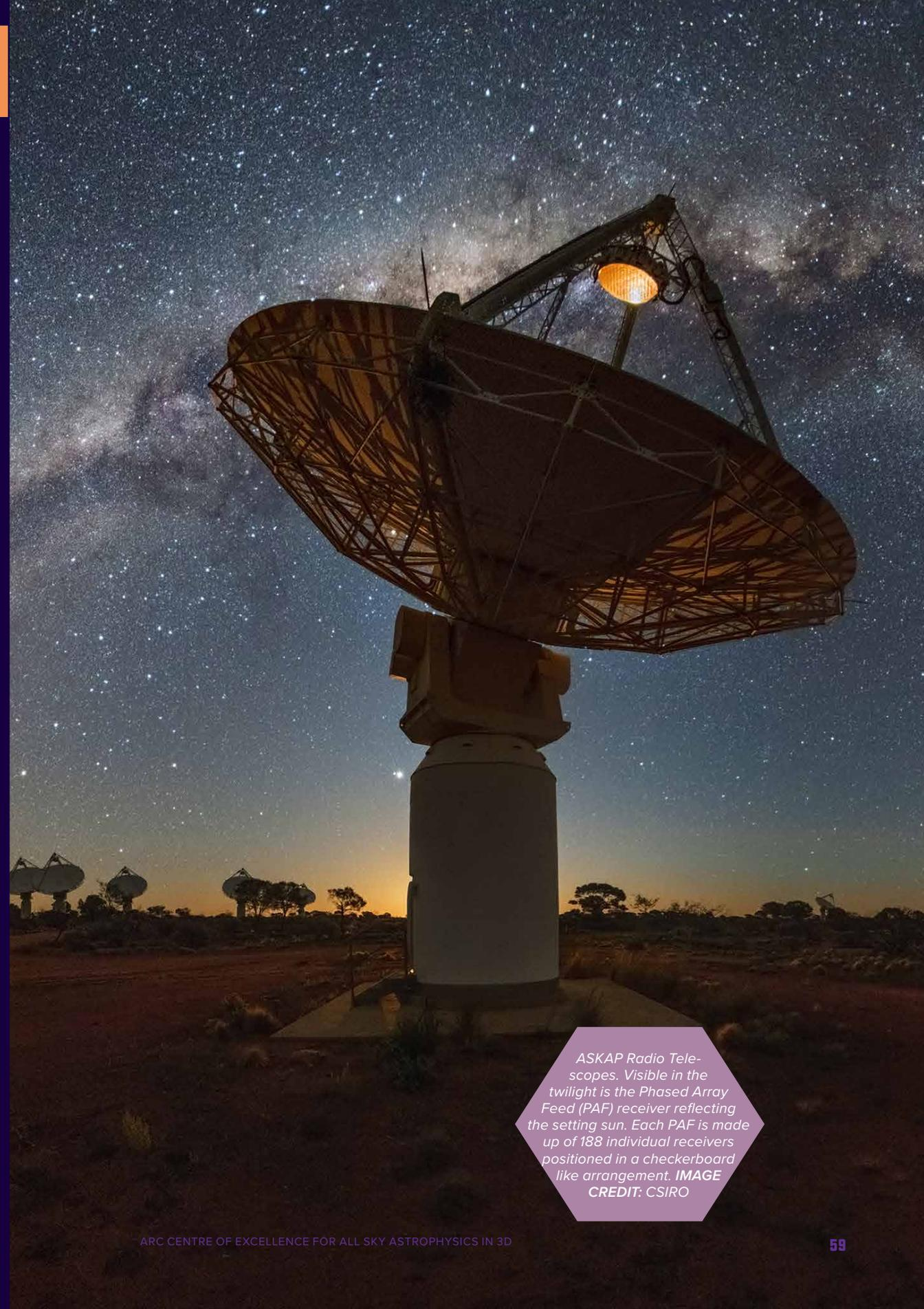
*ASKAP Radio Telescopes. Visible in the twilight is the Phased Array Feed (PAF) receiver reflecting the setting sun. Each PAF is made up of 188 individual receivers positioned in a checkerboard like arrangement. IMAGE CREDIT: CSIRO*
