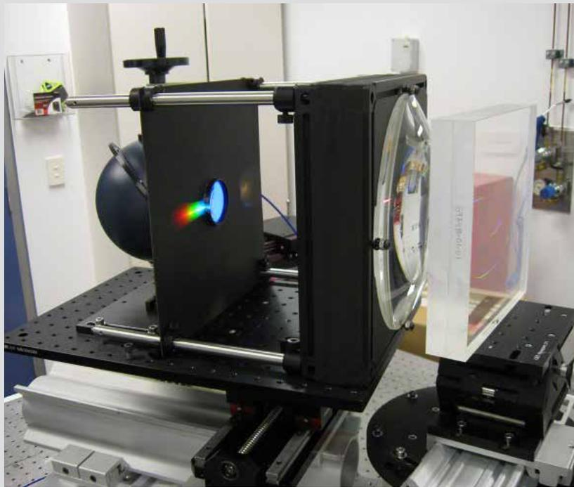
*The Hector spectrograph VPH grating being tested at AAO-MQ in Sept 2020.*
