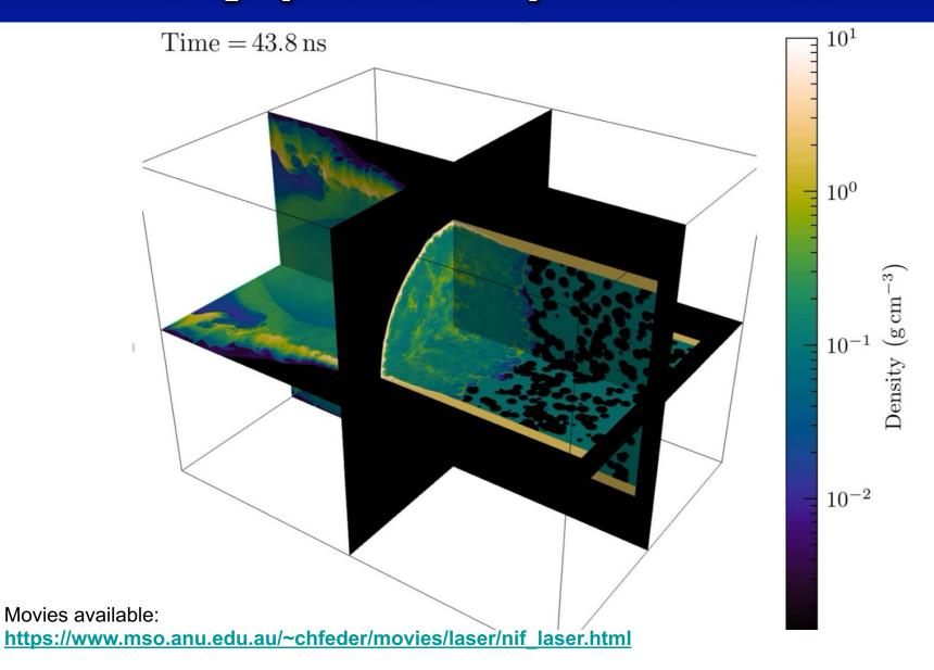
Simulation of a laser-induced shock running into foam
