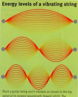
Pluck a guitar string and it vibrates as shown in the top panel at its longest wavelength (lowest pitch). The string can also vibrate at higher pitches, as shown, which have their own wavelengths, much as an electron in an atom has fixed energy levels. Both can take certain values, both have a minimum energy level (like the longest wavelength of the string). At its lowest energy the electron can't lose energy, so atoms do not collapse.
