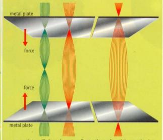
or zero-point oscillations (quantum fluctuations of particles coming into and going out of existence) to occur. In this diagram the two vibrations shown at left can occur between the plates. The vibration at right, however, is too long to occur inside the plates (but still occurs outside the plates). The net effect is a greater pressure on the outside of the plates (because there are fewer vibrations between the plates).
