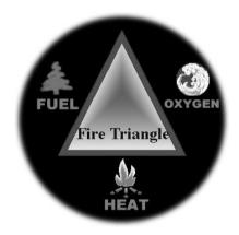
Essentially, Fire extinguishers put out fire by taking away one or more elements of the "FIRE TRIANGLE"
