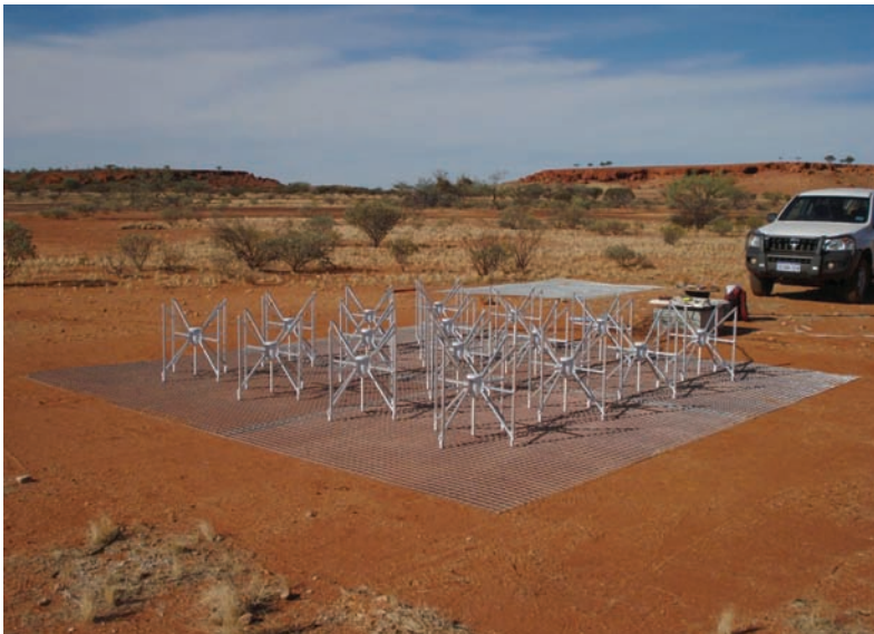
Left: An MWA antenna 'tile' being field tested in the outback of Western Australia.
