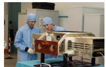
Under development, a wide-field imager instrument for the SkyMapper telescope being built for RSAA's Siding Spring Observatory.
