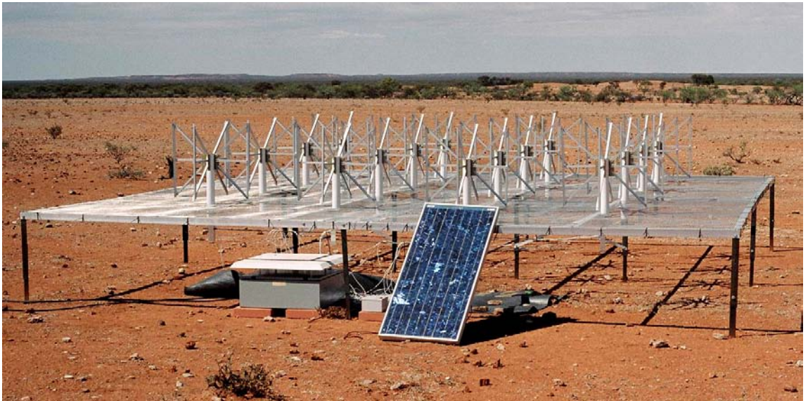
Above: An antenna "tile" with beam former, and solar panel on site at Mileura Station, WA. Coaxial cables run to left to a caravan containing the receiving system.
