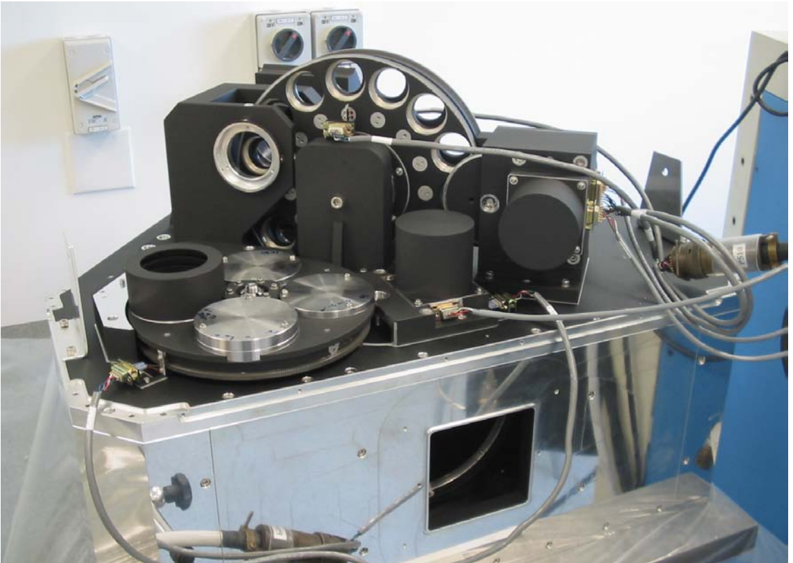
Above: The GSAOI camera before installation in the GSAOI cryostat. Light enters through the dark square (lower center) and is directed through the two large filter wheels (upper center) and ultimately through the smaller wheel (left) to the detector mosaic. The whole camera operates at a temperature of -210^{\circ}\text{C} to optimize performance.
