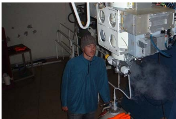
Above: Grant Kennedy refilling the detector dewar on the 40inch telescope with liquid nitrogen.
