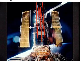
The radiation bounces off a secondary mirror (suspended high), and passes through a hole in the middle of the primary mirror. Detectors and instruments are placed down here behind the primary.
