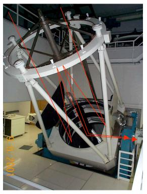
bounces off another two mirrors and goes through the hinge in the other axis. This means that the light can be sent to the same place regardless of where the telescope is pointing. You can thus build extremely large and stable instruments, such as echelle spectrographs here. The price you pay is 6 or more reflections, each of them costing you light.
