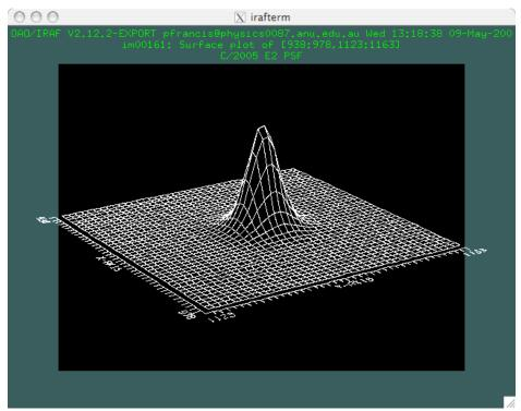
This is a nice normal "point spread function" or PSF. The PSF shows how the light from something that is really a point (such as a star) is smeared by seeing and the telescope optics. Here is a radial plot:
