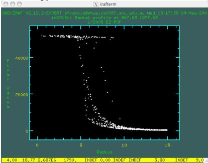
This star, though not bleeding so dramatically, has clearly saturated the CCD (hence the flat topped profile), and is also useless for measuring brightnesses.
