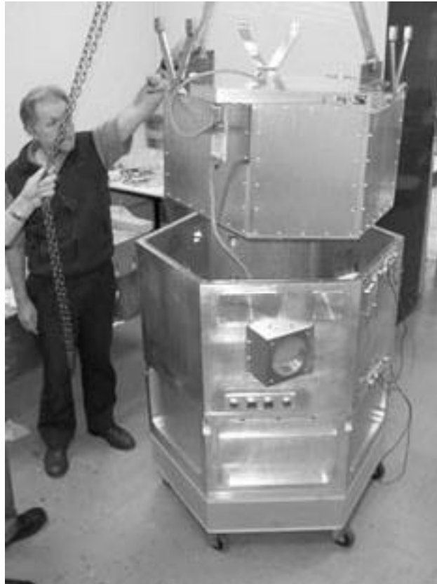
Peter Conroy supervising the installation of the NIFS cold work surface plate and radiation shields in the NIFS cryostat prior to the first cooldown.
